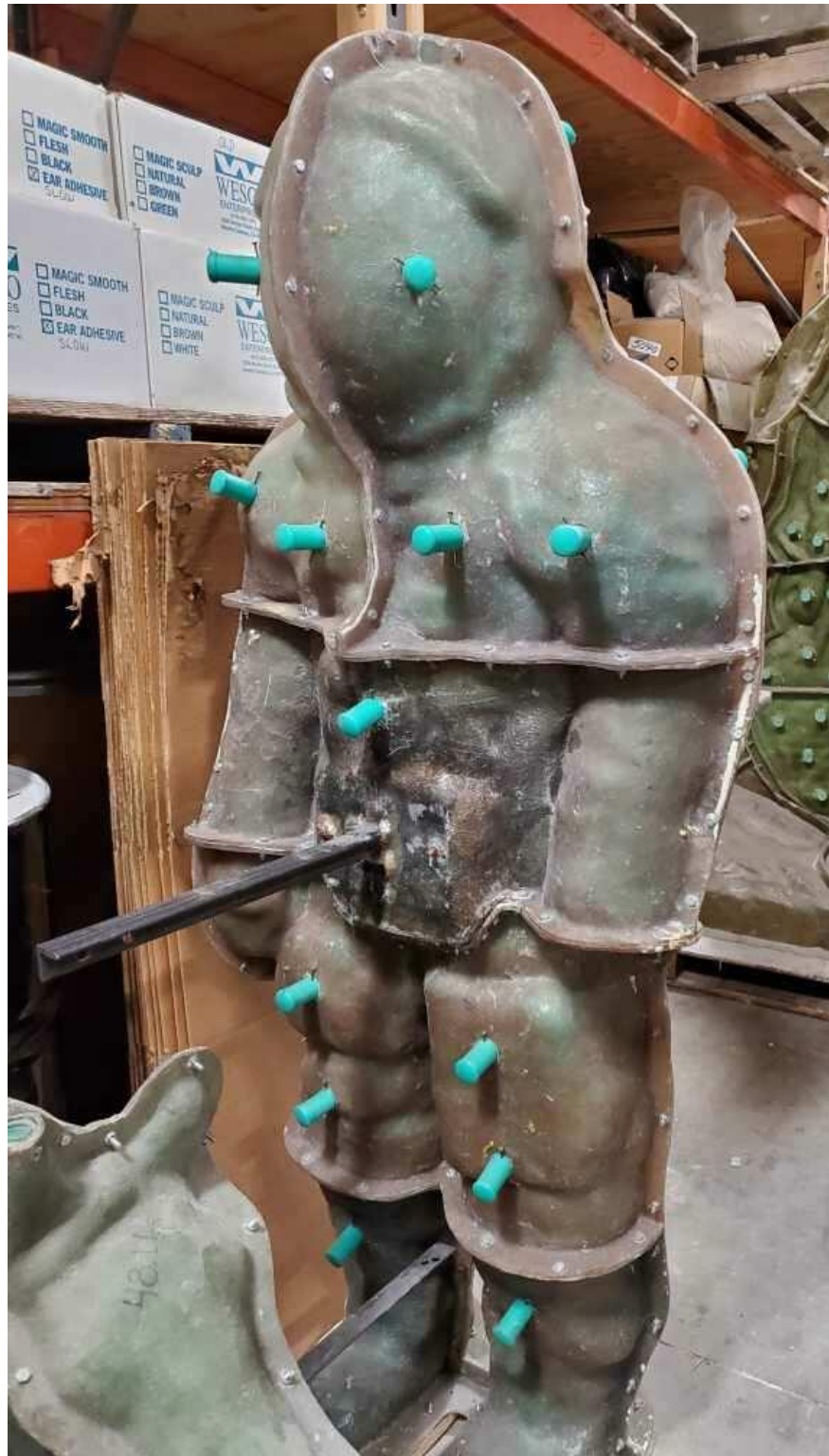
A Mold was Created from the 3D Print to Facilitate Roto-Casting
